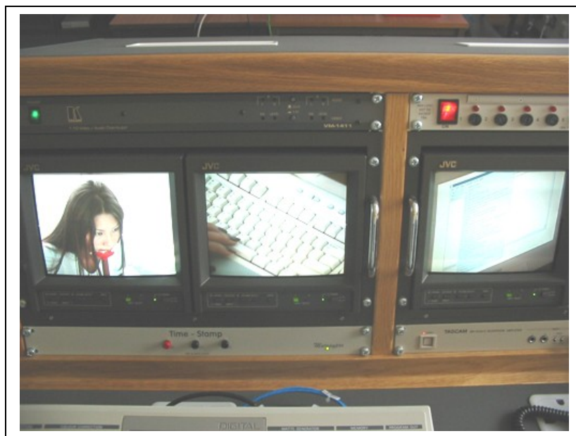
Figure 15 Monitoring console equipped with three CCTV cameras, used to observe participants
