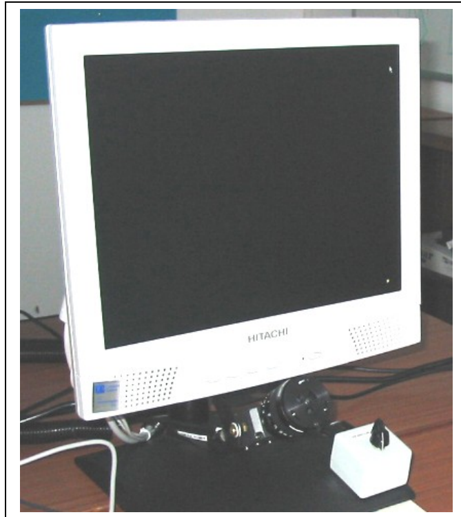
Figure 12 The eye tracker used in the present study: a desktop computer with an infrared camera mounted beneath the monitor.
