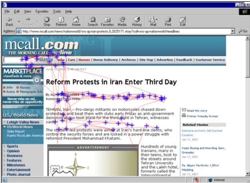
Figure 18 An example of “absolute drift” in the eye movement record: every gaze point has drifted in the same direction by the same amount.
